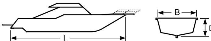
**Note:** **D** is normally measured from the deck edge down to where the hull meets the keel, except for vessels designed for sailing where the interface between the “keel” and the “bottom skin of the hull” is not clearly defined (as is the case with an “integral” or “faired” keel), for which the depth is measured to the bottom of the keel.
